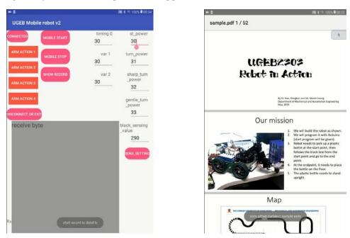
Figure 2: Screenshots of the developed tablet application: In manipulating mode and in manual mode, respectively.
