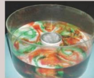
Weather in a Tank for geophysical fluid dynamics (GFD) experiment using a rotating tank
