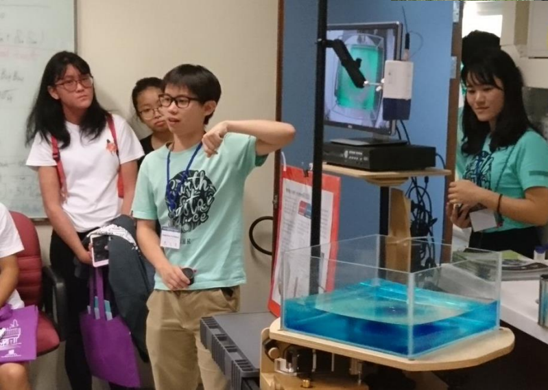
Weather in a Tank for geophysical fluid dynamics (GFD) experiment using a rotating tank
