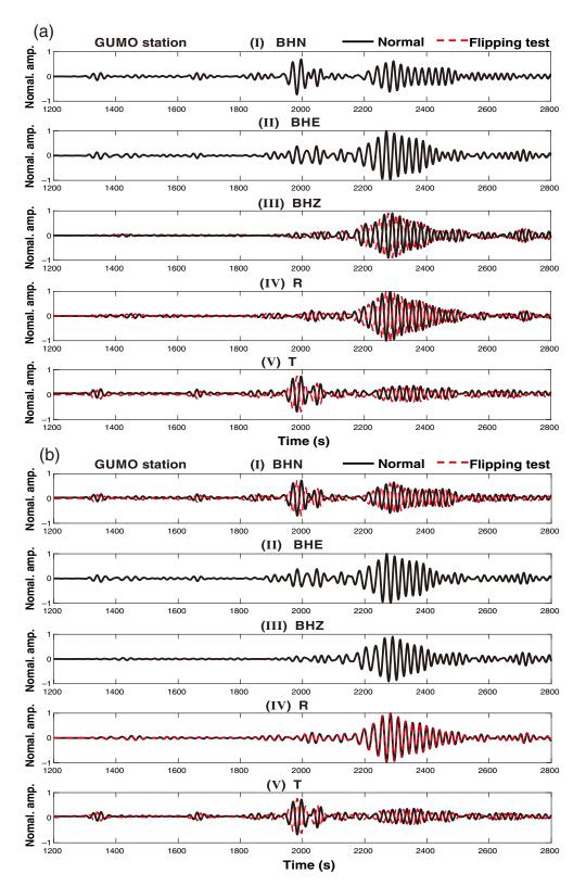
Figure 6. Testing effects of polarity reversal on orienting radial (R) and tangential (T) components using the GUMO station. Effects of (a) vertical polarity reversal and (b) one horizontal polarity reversal on analysis of Rayleigh-wave polarization and oriented R and T components. Information of the earthquake: original time 8 December 2016 14:49:45, latitude = 40.4535°, longitude = -126.1936°, event depth = 8.5 km. The color version of this figure is available only in the electronic edition.
