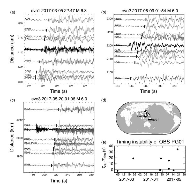
with different origin time, azimuth, and known Global Centroid Moment Tensor (Global CMT) solutions. After inspecting waveforms of earthquakes with clear *P* arrivals, we found that the vertical polarities of OBS stations remained reversed during the entire deployment. Such polarity reversal does not affect earthquake detection or location but inevitably influences the estimates of horizontal orientations.
