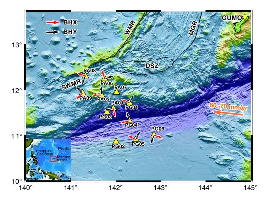
**Figure 2.** A map of OBS (yellow triangles) locations in the southern Mariana. Red and black arrows indicate the estimated orientations of BHX and BHY components, respectively. (Inset) Location of the study area (red frame). DSZ, diffuse spreading zone (Martinez et al., 2018); MGR, Malaguana—Gadao ridges; SWMR, Southwest Mariana rift; WMR, West Mariana ridge. The color version of this figure is available only in the electronic edition.
