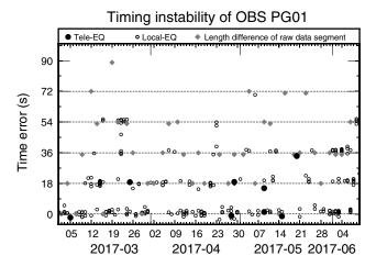
**Figure 4.** Time differences between the observed and theoretical arrivals of OBS PG01 station based on eight teleseismic earthquakes (black dots) and local earthquakes (open dots). Gray diamonds show the length differences of raw data segments relative to normal length. EQ, earthquake.
