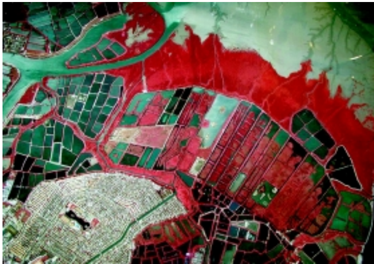
Mapping of Mai Po Marsh by the Aerial Infra-red Remote Sensing Technique.
