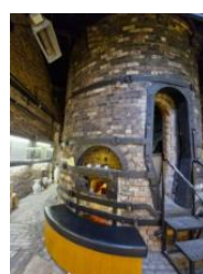
烧陶器的 Bottle Kiln（右侧的已成为博物馆展品） A bottle kiln for firing pottery (the one on the right has been preserved as a museum exhibit)
