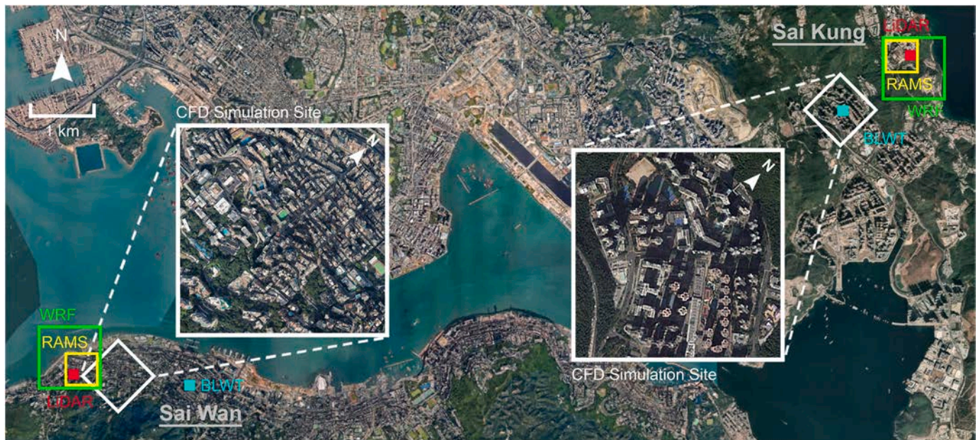
Fig. 2. Two selected high-density urban sites (800 m × 800 m) in Hong Kong for reproducing vertical wind speed profiles, and the locations of nearby ground-based wind LiDAR, as well as the corresponding source points/cells for estimating vertical wind speed profiles by conventional methods (i.e., BLWT, RAMS, and WRF).
