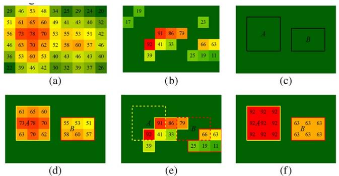
Fig. 2. Illustration of the object-based fusion approach, in which two building height estimates from both stereo and SAR images are combined to generate a fused result. (a) Initial height estimates obtained from stereo images (unit: meters). (b) Initial height estimates obtained from SAR images (unit: meters). (c) Prior building footprints. (d) Extracted height estimates (stereo). (e) Extracted height estimates (SAR). (f) Fused result.
