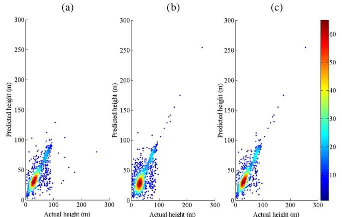
Fig. 4. Scatterplots of the predicted results compared with the actual building height, where the colors indicate the density of the points. (a) Result using the stereo images. (b) Result using the SAR images. (c) Fused result with the proposed approach using both the stereo and SAR images.
