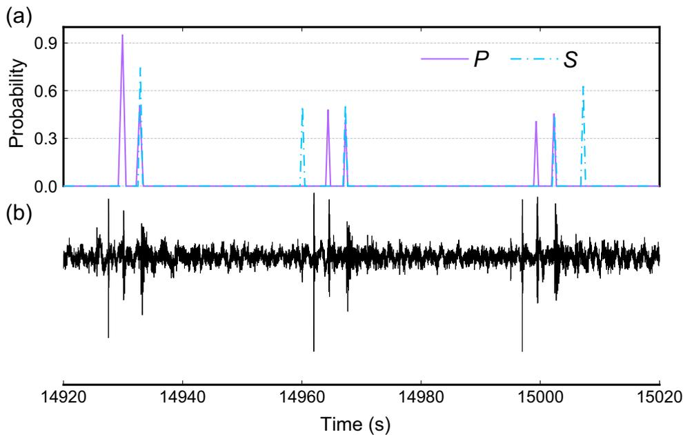
**Figure 4.** False positives predicted by PhaseNet. (a) The probability of  $P$  and  $S$  picks. (b) The impulsive waveforms generated by air gun sources. The color version of this figure is available only in the electronic edition.
