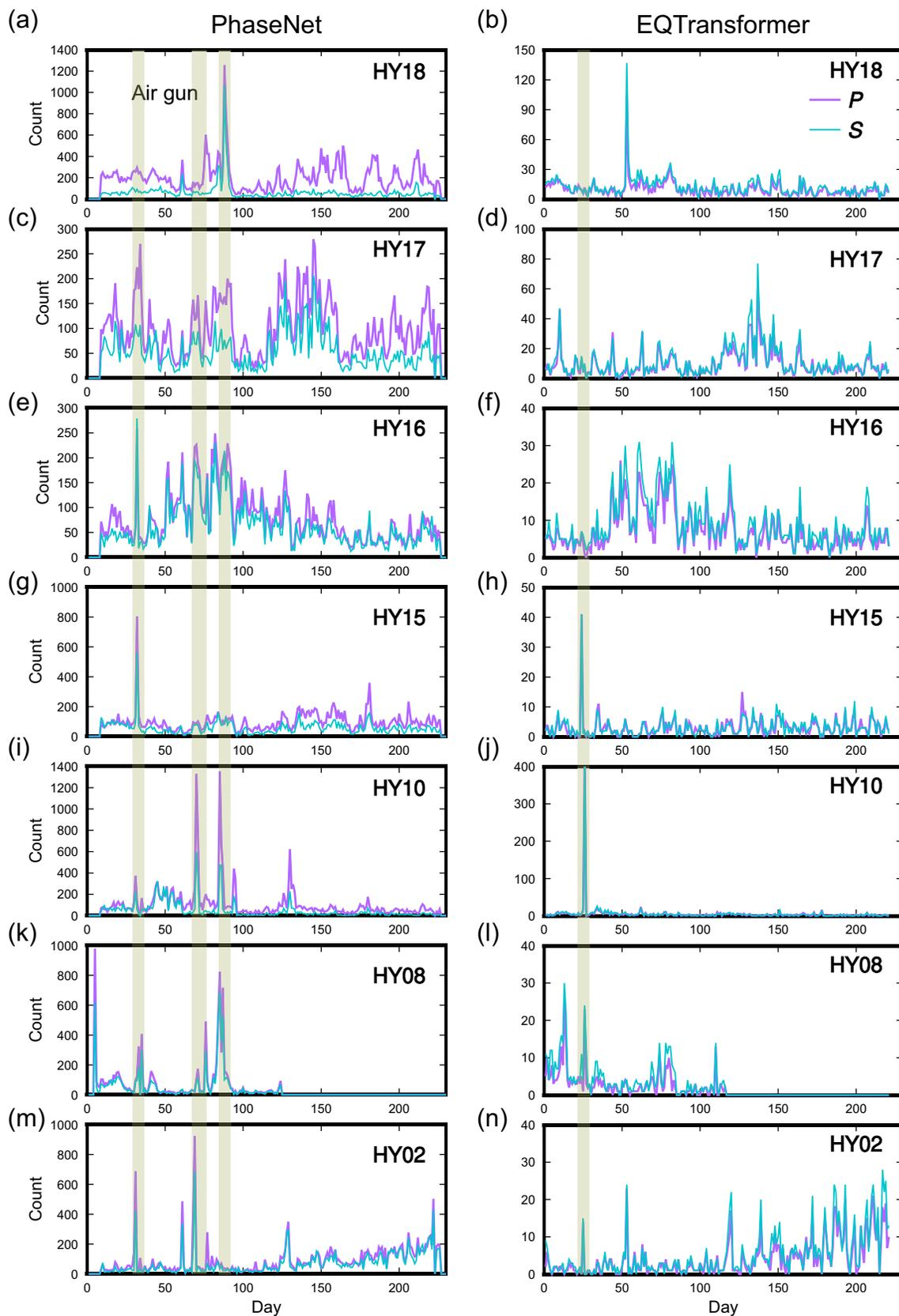
**Figure 3.** The daily number of predicted  $P$  and  $S$  phases on each station by (a,c,e,g,i,k,m) PhaseNet and (b,d,f,h,j,l,n) EQTransformer. The vertical light green bars mark the days with
