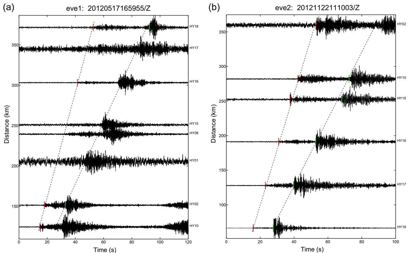
**Figure 7.** Waveforms of two relocated events: (a) event 1 near Zhongnan Fault zone and (b) event 2 at east of the trench, for which locations are marked as stars in Figure 8a. The red and
