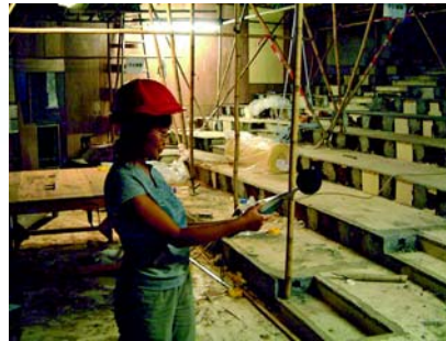
The USEO staff always measures the environmental noise level and occupational noise level of the construction sites and renovation works.
